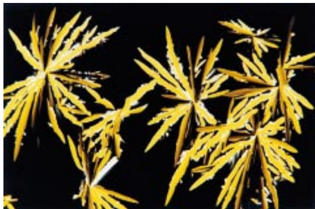
Figure 1. Representative optical polarized texture exhibited by the hexagonal columnar ( \Phi_h ) mesophase of 8 obtained upon cooling from 97 to 94.4 °C at 1 °C/min.
